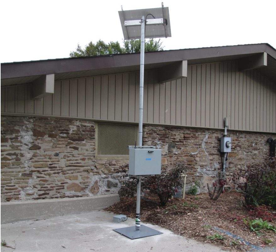
Figure 1. The geophone system and the historical building to be monitored.
